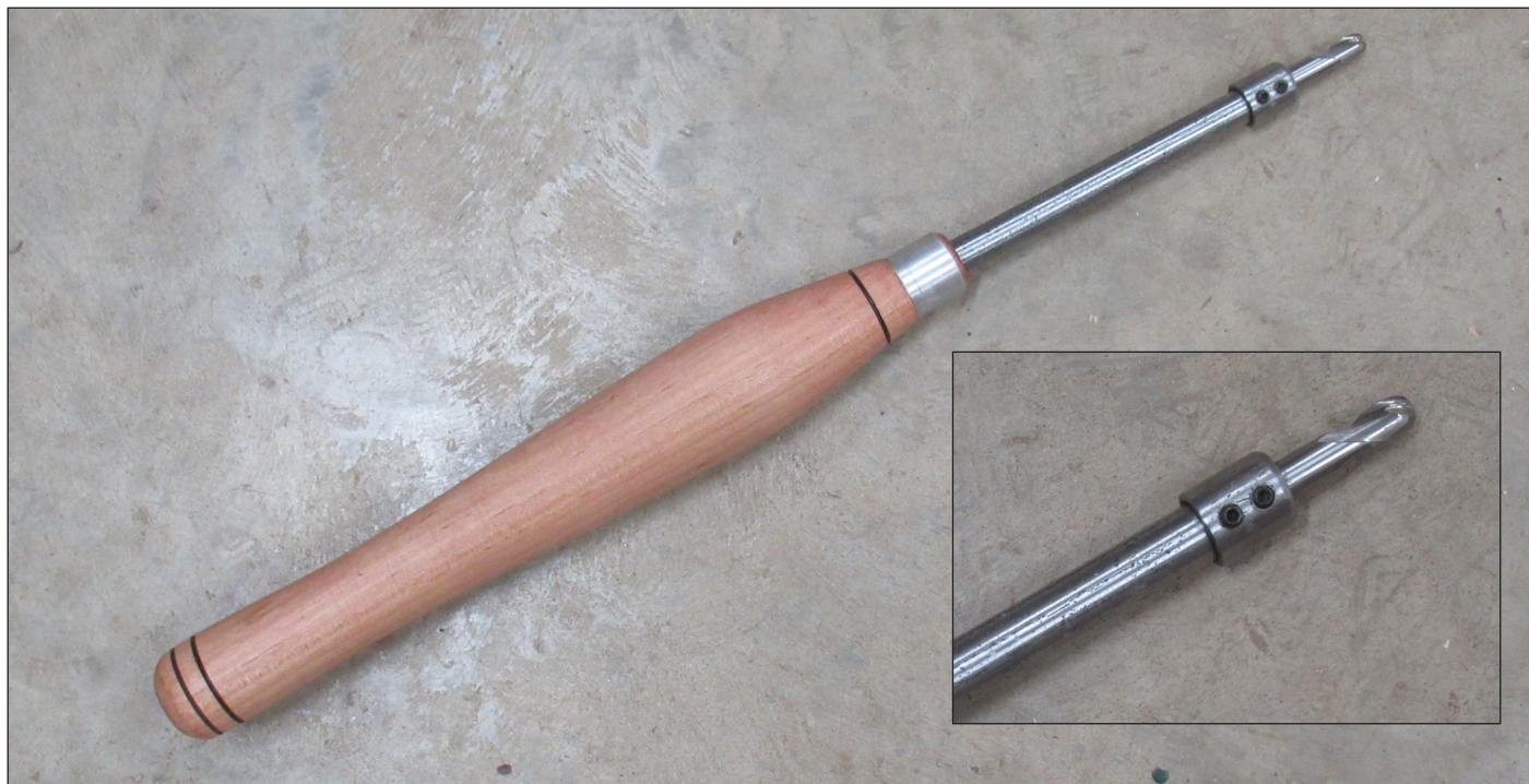
Jim Duxbury shared his new 3/8" ball end mill cutter tool. "I used a piece of 3/8" black steel pipe and a coupling to make it rather than drilling into the end of a solid steel bar. So far it is working great."
