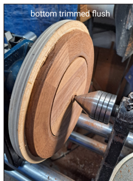
glue ring over sanded floating bottom
