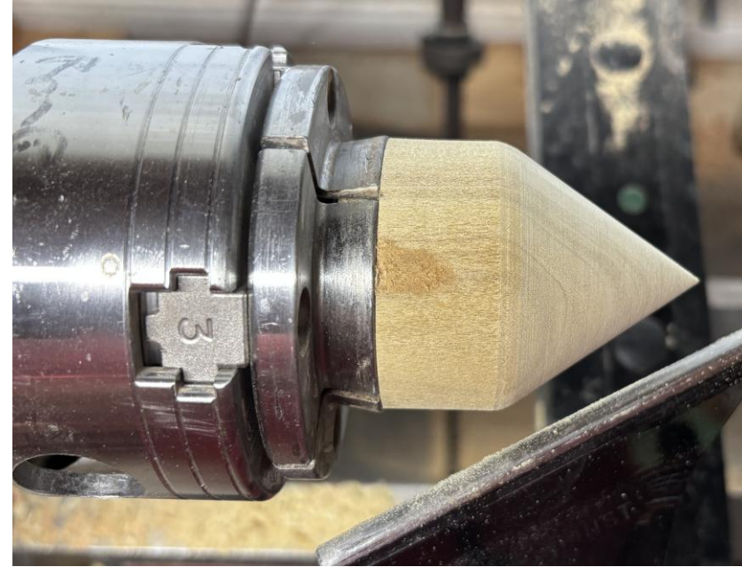
Mount in 4 jaw chuck and turn cone shape
