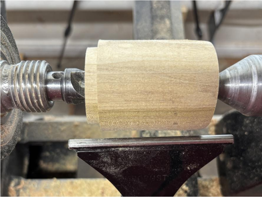
Mount Sanding Jig Blank and turn tenon on one end
