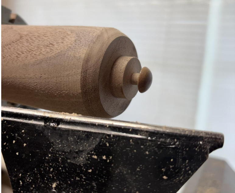
Turn plug dome shape and part off
