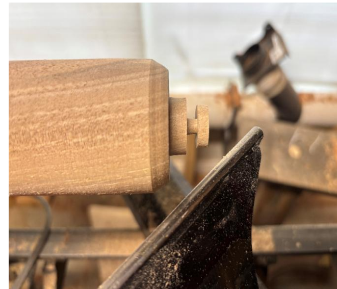
Reverse mount blanks and turn tenon and plug
