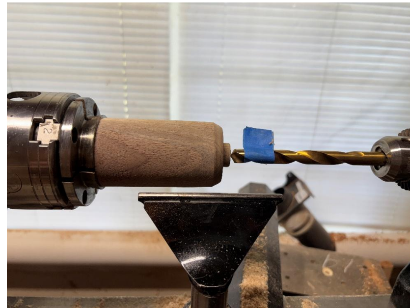
Drill hole for LED light base
