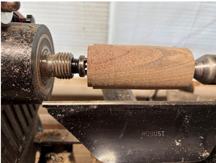
Mount mushroom/plug blank and turn tenon
