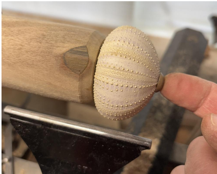
Turn tenon for bottom hole and test fit
