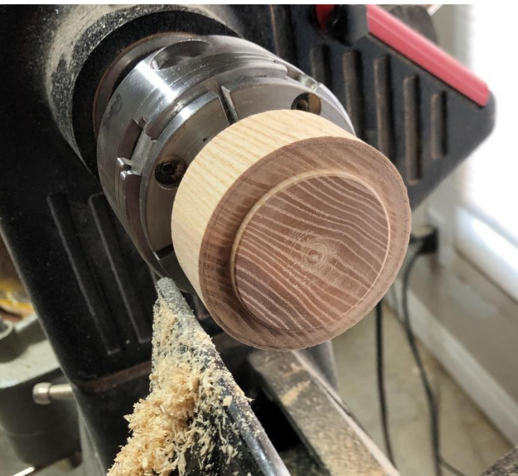
Measure base OD and cut tenon: ~ 53mm
