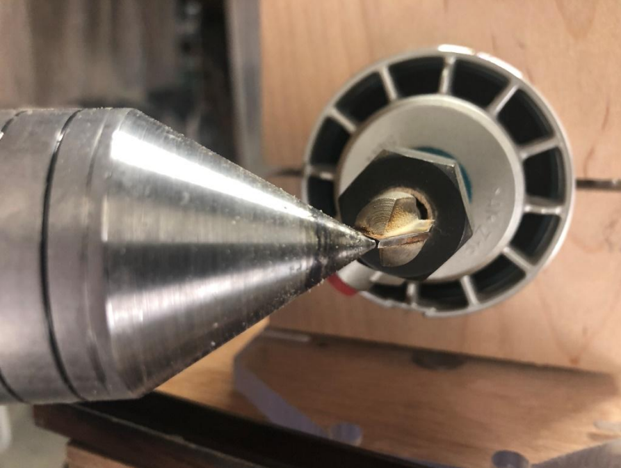
Align router bit to lathe centerline
