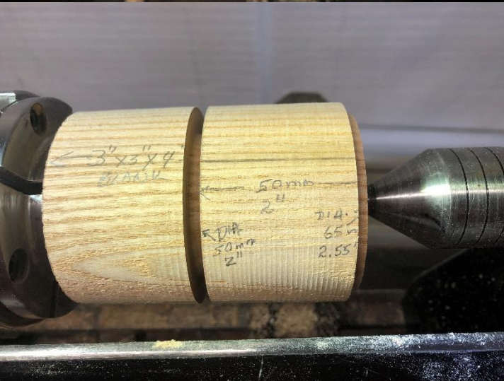
Base: Parted top and bottom diameters
