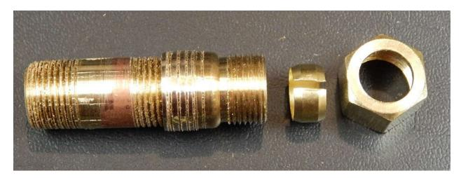
Bore a hole large enough to accept the nipple and adapter in the end of your handle about 1-1/2" deep. The hole should be as snug as you can make it.
